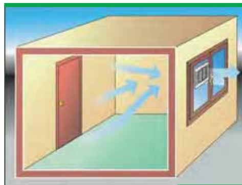
The diagram above shows how extractors work by extracting air from the surroundings and replacing it with cleaner air.
